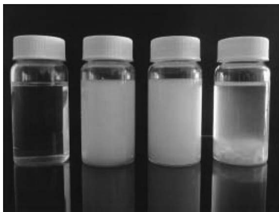
Figure 4. Solvent test of PLA/PA 610 blends with different ratio of epoxy resin (from left to right, 0 phr, 1 phr, 3 phr, and 5 phr).
